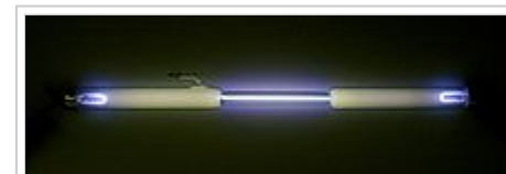
Oxygen discharge (spectrum) tube. The green color is similar to the color of an "aurora borealis"
