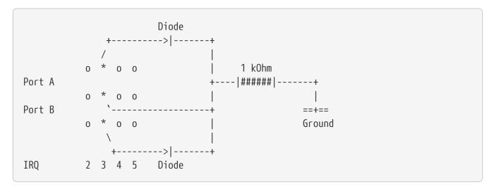
The cathodes of the diodes are connected to a common point, together with a 1 kOhm pull-down resistor. It is essential to connect the resistor to ground to avoid floating of the IRQ line on the bus.
